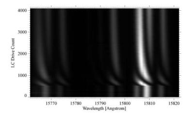
*Figure 3.* The transmission of the thickest module  $M_1$  as a function of drive voltage V and wavelength  $\lambda$ . The retardance of LCVR does not have any response in the range of 0–500 counts. The *horizontal slices* along the x-axis present the transmission profiles under different drive voltage. The *vertical slices* along the y-axis present the calibration curves as transmission vs. drive voltage under 32.0 °C.
