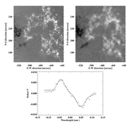
*Figure 6.* Magnetograms of NOAA AR 10781 obtained by IRIM at 16:02 UT (*left*) and MDI at 16:00 UT (*right*). (*Bottom panel*) Stokes V profile and its fitting of an interesting small-scale magnetic structure. The fitted intrinsic field strength is 482 G with a filling factor 49.3%, and the corresponding true magnetic flux is  $2.04 \times 10^{17}$  Mx on an area of 206 km  $\times$  206 km.
