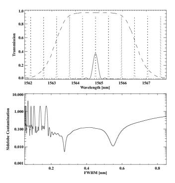
*Figure 2.* (*Top*) Transmission profiles of the birefringent filter (*solid curve*), the FPI (*dotted curve*), and the interference filter (*dashed curve*). (*Bottom*) Contamination from sidebands as a logarithmic function of FWHM of the birefringent filter bandpass. A contamination as low as 0.53% can be obtained with a FWHM approaching 2.744 Å.
