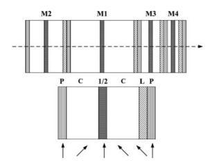
*Figure 1.* Optical diagram of the NIR narrow-band tunable birefringent filter. The upper half of the figure shows the scheme of four birefringent modules marked by  $M_1$ ,  $M_2$ ,  $M_3$ , and  $M_4$ . The lower half shows the detailed optical configuration of a single tunable wide field module. *P*: polarizer; *C*: Calcite; 1/2: half waveplate; *L*: LCVR; *arrows* represent the direction of optical axis for each optical element.
