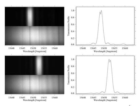
*Figure 4.* The calibration results and transmission profiles when tuned to Fe I 15648.5 Å and Fe I 15652.9 Å spectral lines. (*Left panel*) The transmission bandpass of the spectrograph including or excluding the filter system in the calibration optical path. (*Right panel*) The corresponding transmission profiles. The concave centering at the peak shows the core of the spectral line.
